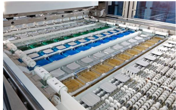
Fig.4: RENA CupCellPlate - single side pseudo inline tool for cleaning and Ni/Cu/Sn plating
